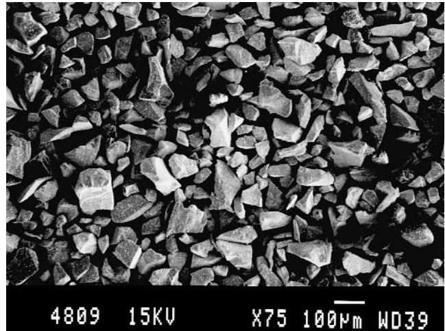
Fig. 2 Scanning electron micrograph of iron ore particles
